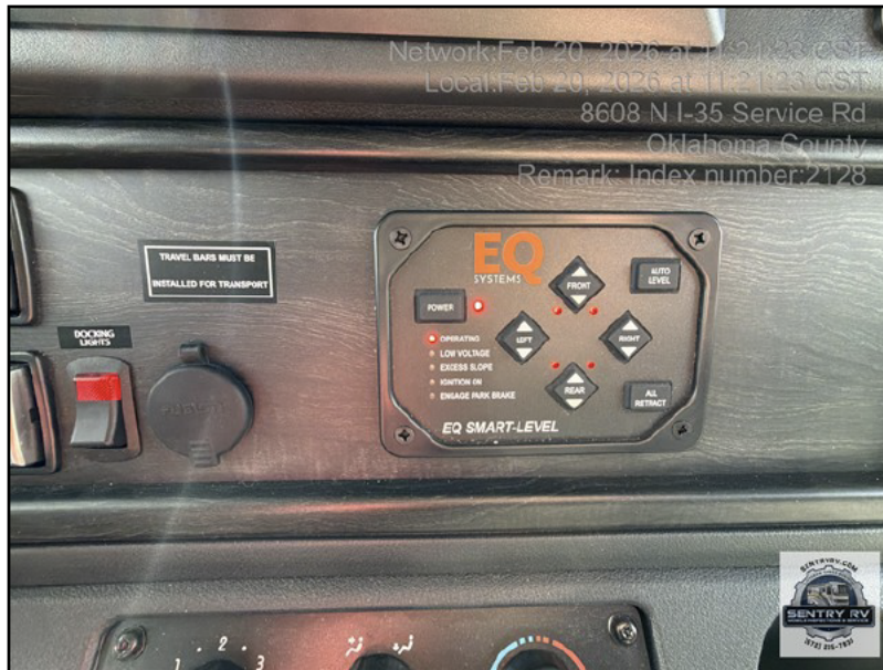
Leveling Control Panel
